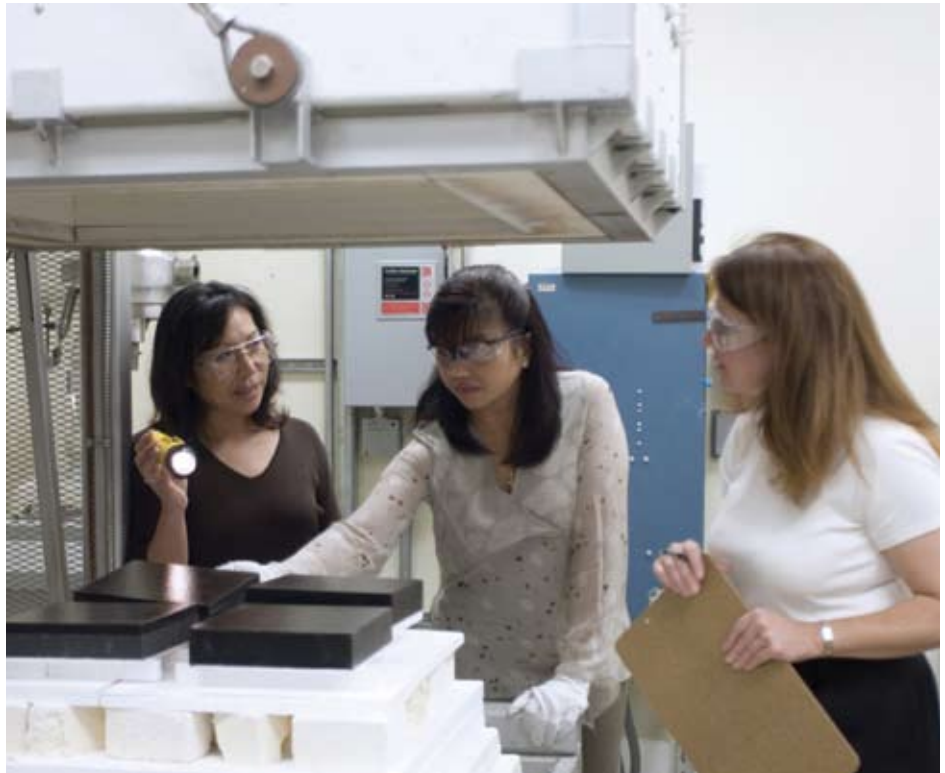
MaryAnn Santos (center) repositions a Boeing Rigid Insulation tile in a high-temperature furnace as she and teammates Vann Heng (left) and Karrie Hinkle complete the coating firing process by inspecting the tiles.
