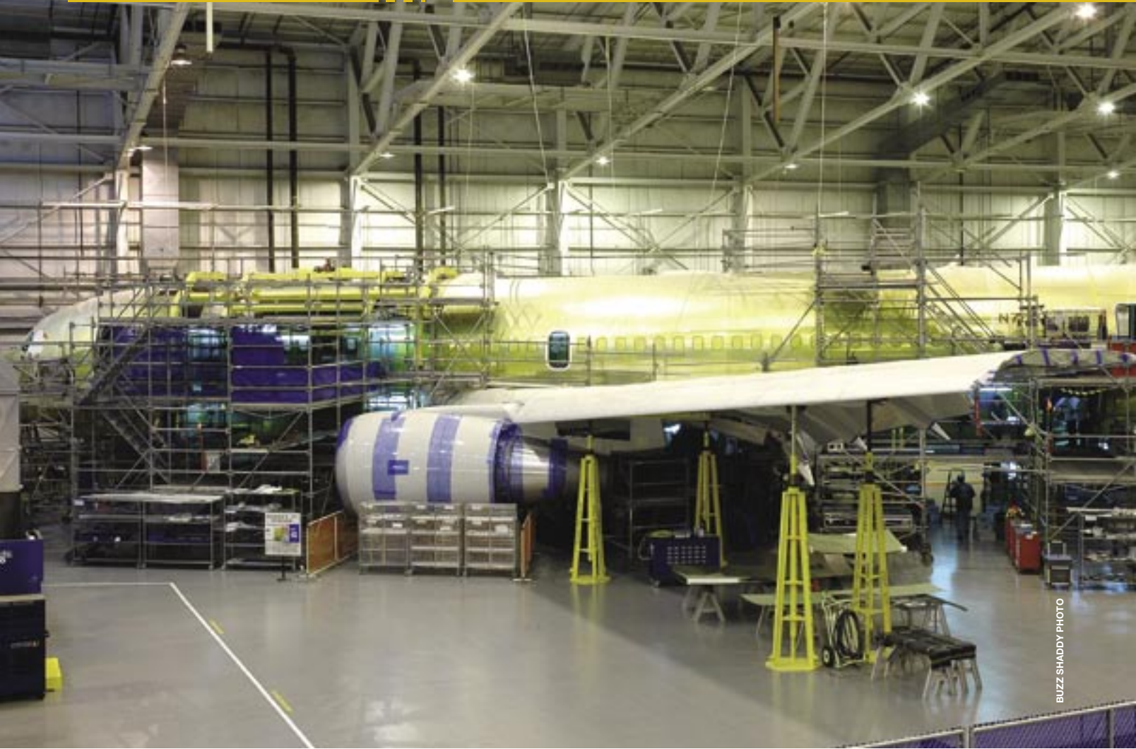
Above: Japan's KC-767 is at the Integrated Defense Systems facility in Wichita, Kan. It will be configured as a convertible freighter, with air refueling boom and Japan-unique avionics requirements. Right: Boeing's Chris Dahl and his colleagues work inside Japan's KC-767, which will be the country's first-ever aerial-refueling tanker.
