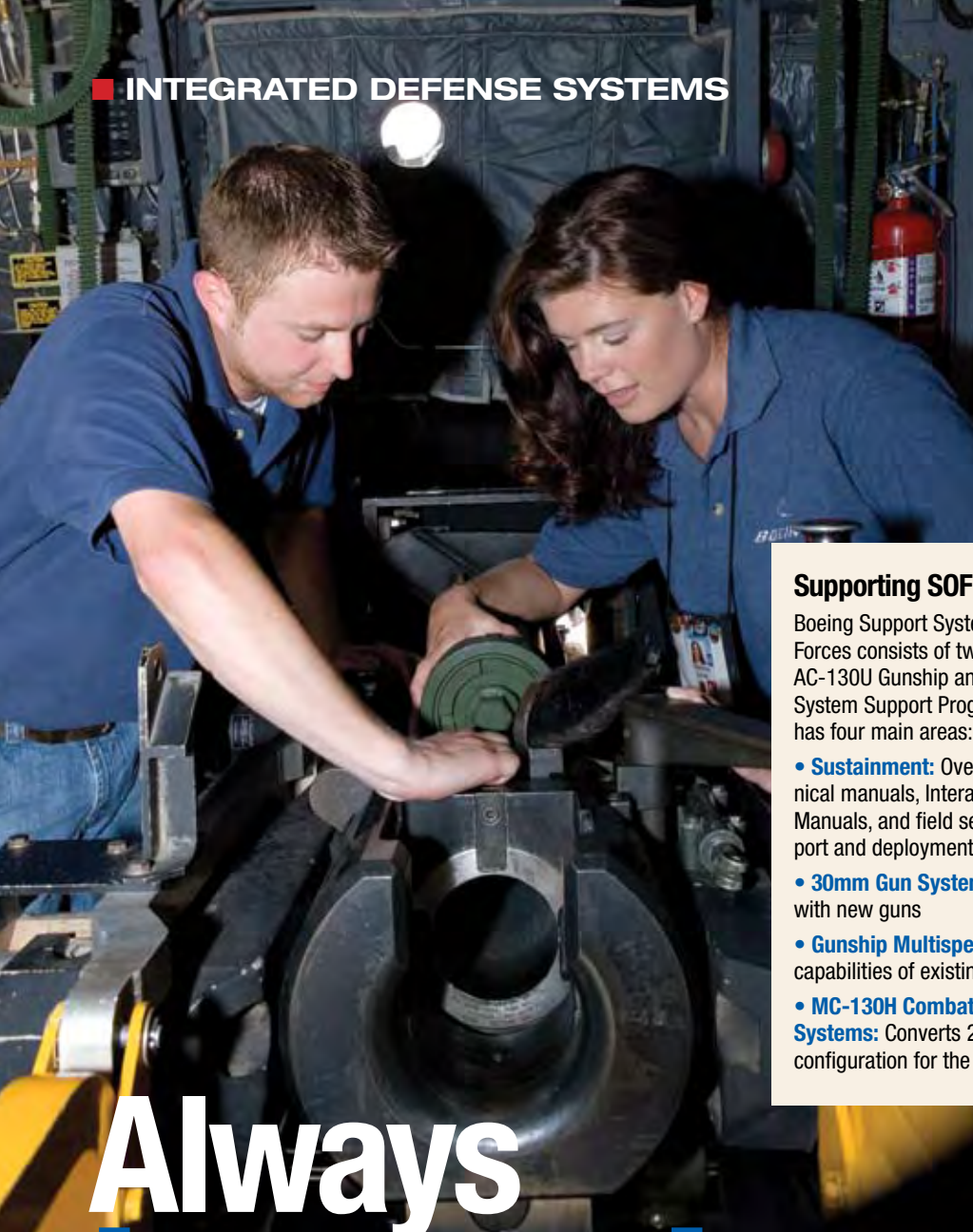
At the U.S. Air Force Special Operations Command headquarters at Hurlburt Field, Fla., Jeremy Mustain and Courtney LaRue, Boeing Special Operations Forces field service representatives, work on an AC-130U Gunship's 105mm gun position.
