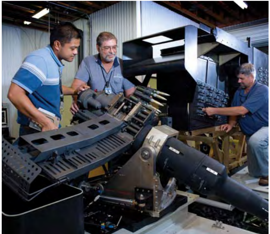
From left, Paul Parinas, Mike Banning and Steve Fick of Boeing Special Operations Forces in Fort Walton Beach, Fla., test the 30mm weapon system, which is loaded on the AC-130U Gunship.
