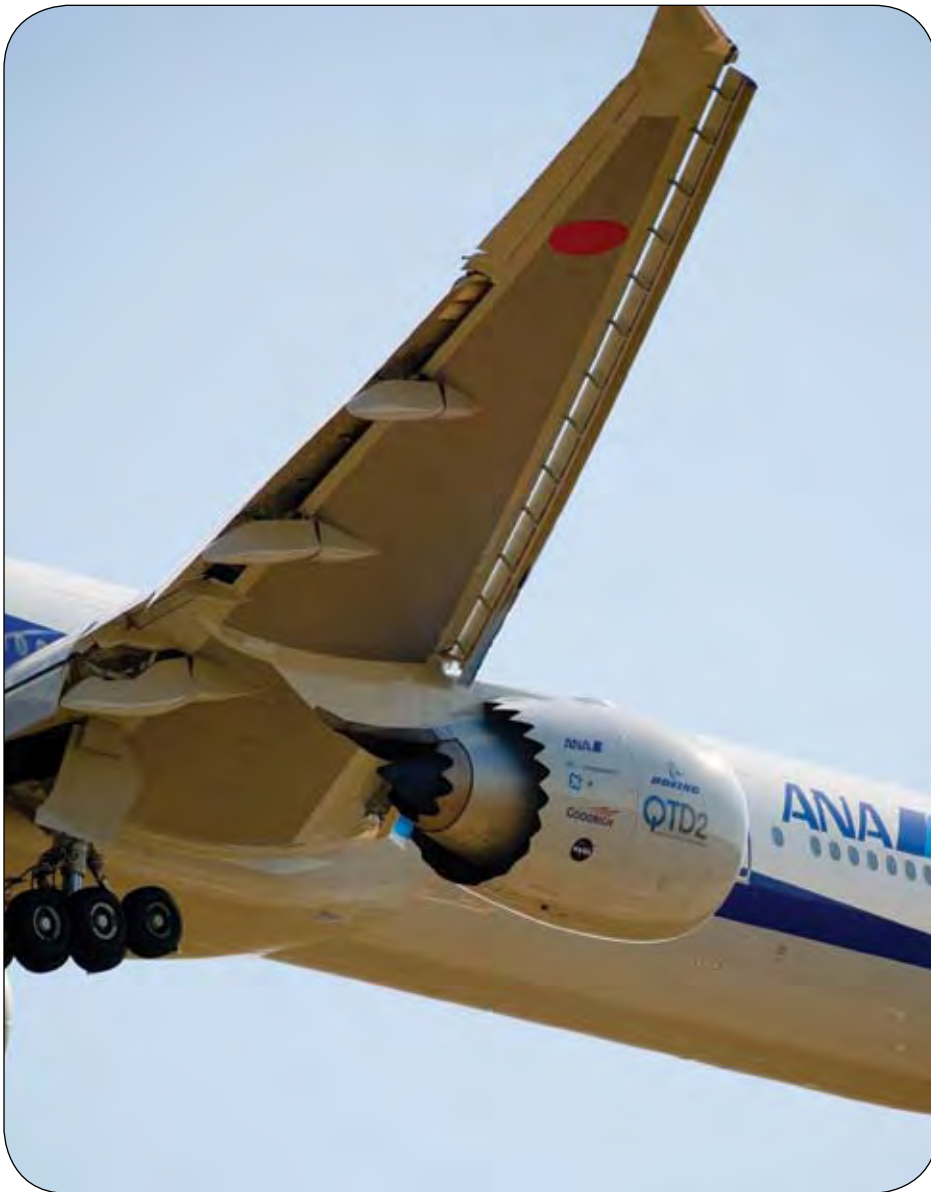
All Nippon Airways last year let Boeing use one of its 777-300ER (Extended Range) airplanes to gather data on airplane noise and test technologies that would help reduce it—such as chevrons seen here at the back of the nacelle and the engine exhaust nozzle.
