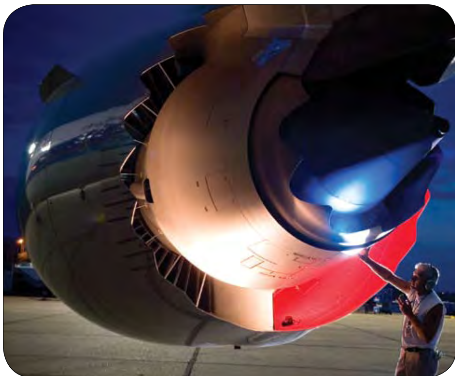
Chevrons, the jagged edges on the rear of engine nacelles, ultimately reduce jet rumble noise for the community during takeoff. Their development represents one of many efforts Boeing is involved in to reduce noise.
