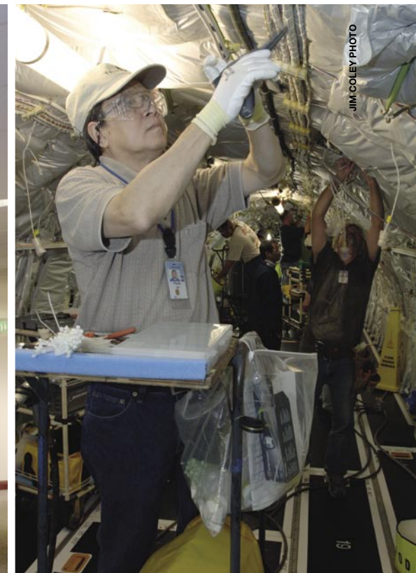
Below right: In the Renton, Wash., factory, Thuan Le ties the overhead Passenger Cabin wiring on a Boeing 737 after clamping is complete.
