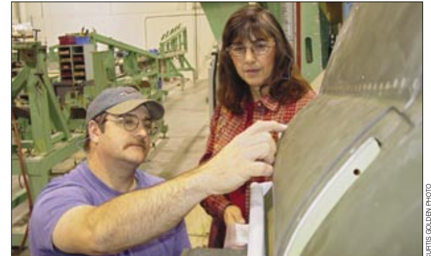
MCALESTER, OKLA. 7:45 A.M. Jerry Williams (left) and Eoline Withers verify hole locations for a detail part on a 747 torque box final assembly. When finished, they will pass this 12-foot-5-inch-by-70-inch assembly to Shipping for travel to the Tulsa, Okla., facility.
